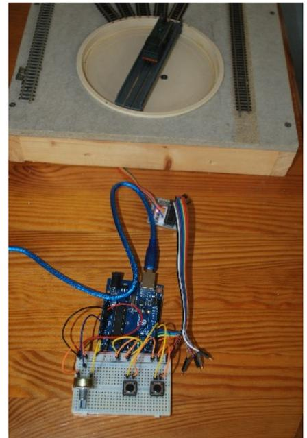
After much experimentation, a final design was decided upon using two buttons to control the clockwise and anti-clockwise rotation of the turntable. It was considered necessary to add a speed controller to ensure that a realistic speed of movement could be established. The program (or 'sketch' as it is called) was written accordingly to operate these functions and uploaded to the micro-controller at the heart of the Arduino board.
